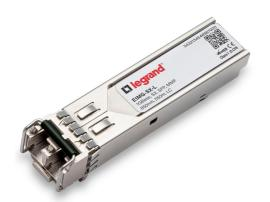
Brocade-Foundry E1MG-SX Compatible 1000Base-SX SFP Transceiver (MMF, 850nm, 550m, LC Duplex, DDM, I-Temp)
