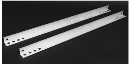
Steel mounts designed to be attached to the outside of the ceiling box and support the box with threaded 3/8'' (9.5mm) diameter threaded rod. Two (2) brackets included.
