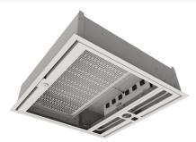
Fully finished enclosure designed to manage and store A/V equipment in an air handling plenum space above a NO ceiling. Equipped with dry contact controlled receptacles that can be switched off when not in use and has a built-in fan to keep the temperature of the equipment cool. Built-in projector mount that utilizes a 1 1/2" standard NFS fitting and is rated to support a load up to 50 lbs.
