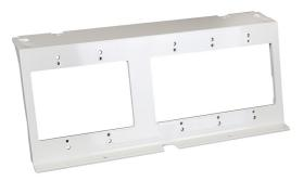
Equipped with one 2-gang standard size device opening and one 3-gang standard size device opening. Accepts a standard 2-gang (4 9/16'' x 4 1/2'' (116mm x 114mm)) and a 3-gang (6 3/8'' x 4 1/2'' (162mm x 114mm)) device plate.
