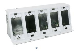
Bank of five (5) compartments that accept power, communications and audio/video devices. Accepts EFB10 Series device plates (2 1/32" x 4 5/8") (58mm x 117mm). Includes one mounting bracket, one back plate, one divider, two (2) end caps and two (2) knockout plates. Device plates sold separately. NOTE: Module will fit on either side of the floor box.
