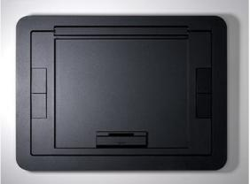
Die cast aluminum cover assembly designed to be used level (flush) with finish floor covering. Available in the following powder coated finishes: black (BK), gray (GY), brass (BS), nickel (NK) and bronze (BZ). For use on Evolution Series 6-, 8- and 10-gang floor boxes (EFB6, EFB8 and EFB10). NOTE: Depth of recess area in plate is 1/4'' (6.35mm).
