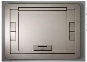
Die cast aluminum cover assembly designed to be used level (flush) with finish floor covering. Available in the following powder coated finishes: black (BK), gray (GY), brass (BS), nickel (NK) and bronze (BZ). For use on Evolution Series 6-, 8- and 10-gang floor boxes (EFB6, EFB8 and EFB10). NOTE: Depth of recess area in plate is 1/4" (6.35mm).
