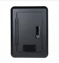
Decorative wall box cover designed to fit onto the 4-gang hinged wall box (EHWB4). Cover comes complete with a hinge that allows the cover to open a full 180 degrees, an integrated handle with lock and key set, and an egress door that allows the cables to exit the box flush against the wall. The cover is offered in two powder-coated finishes white: EHWBC4-WH or black EHWBC4-BK.
