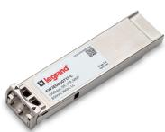
Citrix EW3E0000713 Compatible 10GBase-SR XFP Transceiver (MMF, 850nm, 300m, LC Duplex, DDM, I-Temp)
