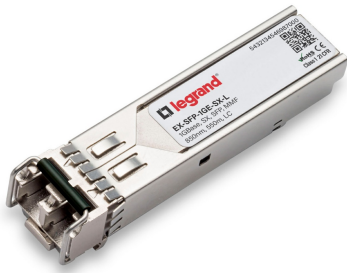
Juniper EX-SFP-1GE-SX Compatible 1000Base-SX SFP Transceiver (MMF, 850nm, 550m, LC Duplex, DDM, I-Temp)
