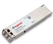
F5 Networks F5UPGXFPR Compatible 10GBase-SR XFP Transceiver (MMF, 850nm, 300m, LC Duplex, DDM, I-Temp)
