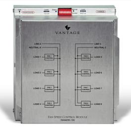
The Wattstopper Architectural Dimming system Fan Module offers an easy and quiet solution for ceiling fan control. This fan module provides control of up to eight different multiple speed ceiling fans. The Fan Module can control four different speed settings plus off.
