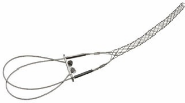
FC075LB: Standard Duty, Closed Mesh, Locking Bale (Universal Eye), Cable Diameter 0.75 - 0.99 inches, Bale Length 18-in, Mesh Length 14-in, Break Strength 1320 lbs.
