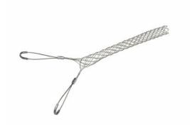
FC125UU: Standard Duty, Closed Mesh, Double -Eye Grip, Cable Diameter 1.25 - 1.49 inches, Bale Length 5-in, Mesh Length 16-in, Break Strength 1920 lbs.
