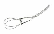
FC150LB: Standard Duty, Closed Mesh, Locking Bale (Universal Eye), Cable Diameter 1.50 - 1.74 inches, Bale Length 18-in, Mesh Length 18-in, Break Strength 1920 lbs.
