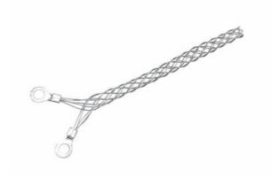
FC22GL: Extra-Hard Use, Closed Mesh, Cable Diameter 0.22 - 0.32 inches, Mesh Length 4.5-in
