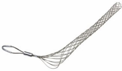
FC2500F: Standard Duty, Closed Mesh, Offset Eye Grips, Cable Diameter 2.50 - 2.99 inches, Bale Length 8-in, Mesh Length 24-in, Break Strength 3760 lbs.
