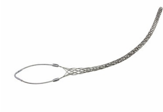
FCHL075U: Standard Duty, Closed Mesh, Single-Eye Grip, Cable Diameter 0.75 - 0.99 inches, Bale Length 10-in, Mesh Length 26-in, Break Strength 2700 lbs.
