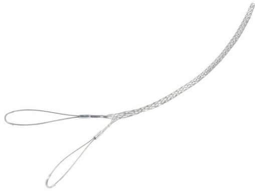
FCHL075UU: Heavy-Duty, Closed Mesh, Double-Eye, Cable Diameter 0.75 - 0.99 inches, Bale Length 10-in, Mesh Length 26-in, Break Strength 2700 lbs.
