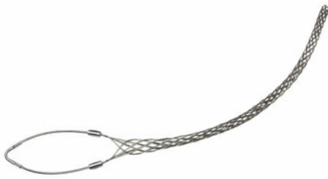
FCHL125U: Standard Duty, Closed Mesh, Single-Eye Grip, Cable Diameter 1.25 - 1.49 inches, Bale Length 10-in, Mesh Length 31-in, Break Strength 4720 lbs.
