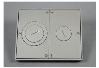
Flangless cover for use in tile or carpet installation. Die-cast aluminum assembly. Provided with one 1" trade size screw plug for power or communication type cabling and one combination 1 1/4" and 2" trade size screw plug for communication type cabling. Allows for feeding both power and communication cabling. NOTE: Add suffix TR to the end of the part number to indicate tamper-resistant cover assembly. Tamper-resistant versions are secured with a single tamper-resistant screw.
