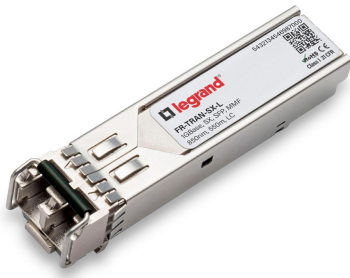
Fortinet FR-TRAN-SX Compatible 1000Base-SX SFP Transceiver (MMF, 850nm, 550m, LC Duplex, DDM, I-Temp)
