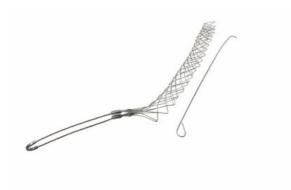
FR100U: Standard Duty, Split Rod, Single Eye, Cable Diameter 1.00 - 1.24 inches, Bale Length 9-in, Mesh Length 15-in, Break Strength 1680 lbs.
