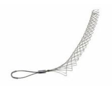
Standard-duty, Split rod, Offset eye. Cable diameter - 1.250-1.490-inch, Bale length - 5-inch, Mesh length - 16-inch, Break strength - 1,680 lbs.
