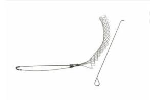
FR175U: Standard Duty, Split Rod, Single Eye, Cable Diameter 1.75 - 1.99 inches, Bale Length 14-in, Mesh Length 20-in, Break Strength 2640 lbs.
