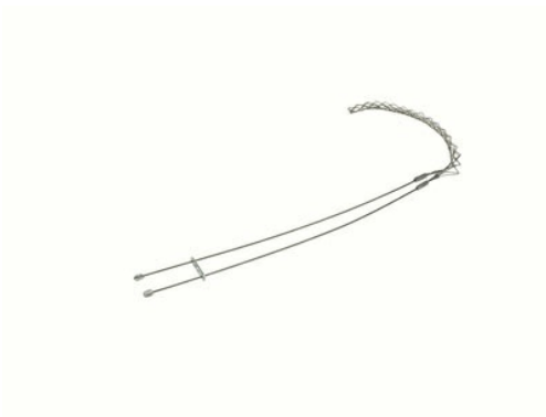
FS062LB: Standard Duty, Split Lace, Locking Bale (Universal Eye), Cable Diameter 0.62 - 0.74 inches, Bale Length 18-in, Mesh Length 11-in, Break Strength 1150 lbs.
