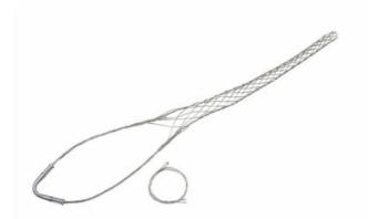
Stainless Steel, Standard-duty, Split lace, single eye. Cable diameter - 0.620-0.740. Bale length - 8-inch, Mesh length - 11-inch, Break strength - 960 lbs.
