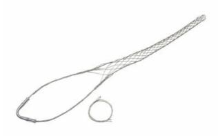
Stainless Steel, Standard-duty, Split lace, single eye. Cable diameter - 0.620-0.740. Bale length - 8-inch, Mesh length - 11-inch, Break strength - 960 lbs.
