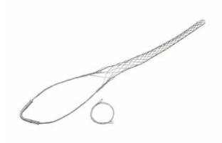
Stainless Steel, Standard-duty, Split lace, Single eye. Cable diameter -0.750-0.990\'\', Bale length - 8\'\', Mesh length - 14\'\', Break strength -1,320 lbs.
