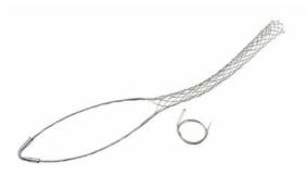
FS150U: Standard Duty, Split Lace, Single Eye, Cable Diameter 1.50 - 1.74 inches, Bale Length 12-in, Mesh Length 18-in, Break Strength 1680 lbs.
