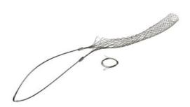
FS250U: Standard Duty, Split Lace, Single Eye, Cable Diameter 2.50 - 2.99 inches, Bale Length 18-in, Mesh Length 24-in, Break Strength 3760 lbs.
