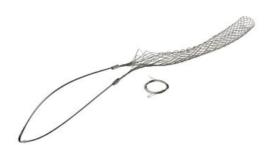
FS300U: Standard Duty, Split Lace, Single Eye, Cable Diameter 3.00 - 3.49 inches, Bale Length 21-in, Mesh Length 26-in, Break Strength 5040 lbs.
