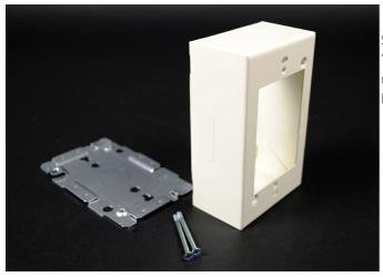
Single Gang Device Box. Cover has twistouts for 2000, 500 and 700 Series Raceways. Base has 1/2'' trade size KO and rectangular KO for extension to wall box. Base has #10 threaded hole for ground connection.
