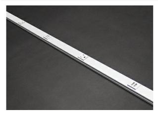
Available in 5' (1.5m) length with 9" spacing. 15A tamper-resistant receptacles. 3-wire, #12 THHN (1 hot, 1 neutral and insulated ground conductor). .040" (1.0 mm) steel housing. Packed two per carton. Each unit supplied with one (1) Coupling and two (2) Blank End Fittings. USB is 2.4 Amps (shared between two ports) 5VDC. Please note the charging load on one module will not affect the charging performance of the other USB modules in the product.
