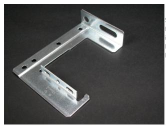
Suspends 3000 Series Raceway from structural ceilings. Designed for use with 3/8" (9.5mm) threaded rod. Hangers should be installed no more than 5" (1.5m) apart along raceway run. This C-Hanger can be mounted back-to-back for double run of 3000 Series Raceway.
