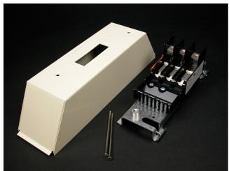
Mounts Square D Quik-Gard QOB bolt-on circuit breakers into 3000 Series Raceway. Rated up to 50A maximum capacity. Includes Square D QON3B Compact Base for single- to three-pole circuit breakers. For GFI breakers, use Square D QOB-GFI Series.
