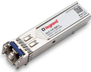
Cisco GLC-LH-SM Compatible 1000Base-LX SFP Transceiver (SMF, 1310nm, 10km, LC Duplex, DDM, I-Temp)
