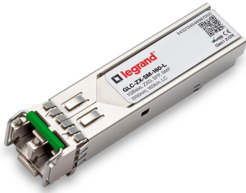
Cisco GLC-ZX-SM-160 Compatible 1000Base-ZX SFP Transceiver (SMF, 1550nm, 160km, LC Duplex, DDM, C-Temp)
