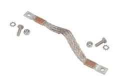
Ground straps provide grounding between spliced runway. Simply pre-drill runway to accept the strap, and connect to runway sections using compression lugs. All compression lugs and .5 in-20 in. Constructed of flexible tinned copper flat braid.
