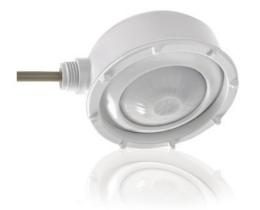
The HBL7W lens is designed for use with the HB3x0W series sensors, which are used in wet locations. It has the same coverage patterns as the dry environment lense, designed for mounting at heights between 20' and 40', with coverage area up to 100' in diameter when mounted at 40'.
