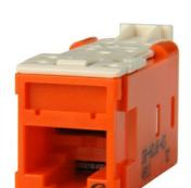
Clarity High Density Jacks (HDJ) unshielded are available in CAT5E, CAT6 and CAT6A, featuring lacing cap termination with icon slot for port ID. Jacks are sold in carton of 20, or bulk pack of 25, termination tool is included with each carton.
