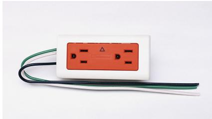
3-Wire 125V NEMA 5-15R orange receptacle. Includes 10 1/2" (267mm) pigtails and inline splice connectors.
