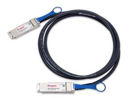
2m Juniper JNP-100G-DAC-2M Compatible 100GBase-DAC QSFP28 to QSFP28 (Passive Twinax Copper, PVC) Direct Attach Cable
