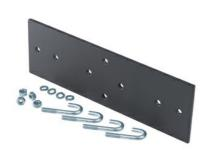
Dimensions: 12 inches H x 7 inches W x .25 inches D Used for junctioning cable runway and equipment racks. Runway can be junctioned parallel or perpendicular to rack. Cable runway mounting brackets mount to the top of the cabinet and provide a surface for attaching 6 in, 12 in, 18 in or 24 in W runway.
