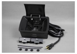
Cord-ended with black, flush cover with decorative recess. Unit comes with two 20A gasketed prewired receptacles with a 12' (3.65m) 14/3 SJT black cord. Includes adapter for Wiremold CM Series Open System communications outlets. Communication modules sold separately.
