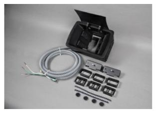
Field-wired with black, flush cover. Unit comes with two 20A gasketed prewired receptacles with a 3/8" (9.5mm) diameter 6' (1.83m) flexible whip. Includes adapter for Wiremold CM Series Open System communications outlets. Communication modules sold separately.
