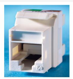
Category 5e Keystone jack, 8-position, 180 degree exit, icon compatible, T568A/B wiring, Package of 25.TechChoice keystone jacks and modules feature an easy-to-follow universal wiring label and support standard termination using a 110-impact tool. The keystone footprint allows for the greatest flexibility in installation scheduling because its rear insertion into the faceplate allows the technician to complete the termination before and during the construction process.
