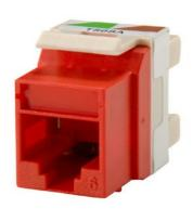
Category 6 Keystone jack, 8-position, 180 degree exit, icon compatible, T568A/B wiring. TechChoice keystone jacks and modules feature an easy-to-follow universal wiring label and support standard termination using a 110-impact tool. The keystone footprint allows for the greatest flexibility in installation scheduling because its rear insertion into the faceplate allows the technician to complete the termination before and during the construction process.
