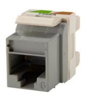
Category 6 Keystone jack, 8-position, 180 degree exit, icon compatible, T568A/B wiring. TechChoice keystone jacks and modules feature an easy-to-follow universal wiring label and support standard termination using a 110-impact tool. The keystone footprint allows for the greatest flexibility in installation scheduling because its rear insertion into the faceplate allows the technician to complete the termination before and during the construction process.
