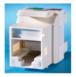
Category 6 Keystone jack, 8-position, 180 degree exit, icon compatible, T568A/B wiring. TechChoice keystone jacks and modules feature an easy-to-follow universal wiring label and support standard termination using a 110-impact tool. The keystone footprint allows for the greatest flexibility in installation scheduling because its rear insertion into the faceplate allows the technician to complete the termination before and during the construction process.
